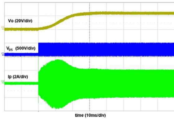
Figure 36. Soft-start Waveforms
