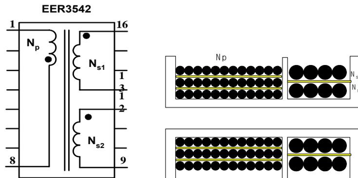
Figure 29. Transformer Structure
