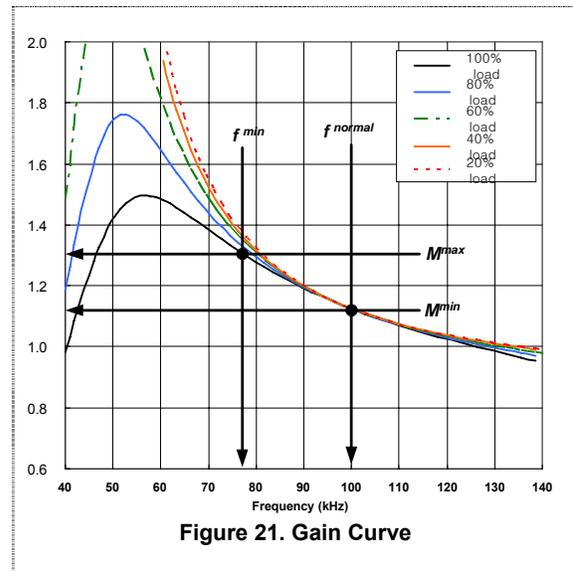
Figure 21. Gain Curve
