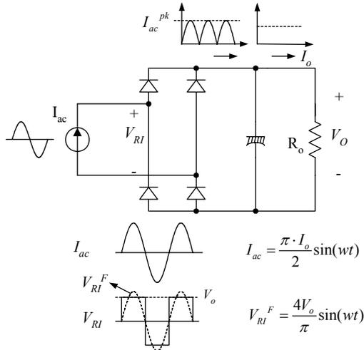
Figure 5. Derivation of Equivalent Load Resistance  $R_{ac}$
