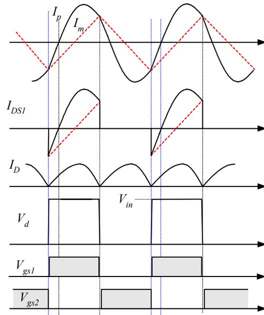
Figure 4. Typical Waveforms of Half-bridge LLC Resonant Converter
