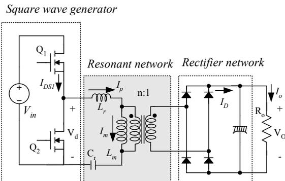
Figure 3. Schematic of Half-bridge LLC Resonant Converter
