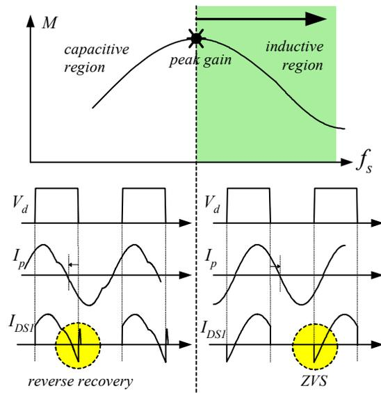
Figure 12. Operation Waveforms for Capacitive and Inductive Regions
