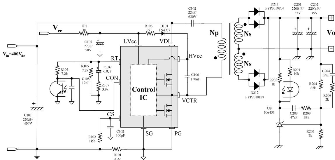
Figure 28. Final Schematic of Half-bridge LLC Resonant Converter
