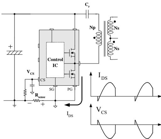
**Figure 26. Half-wave Sensing**
