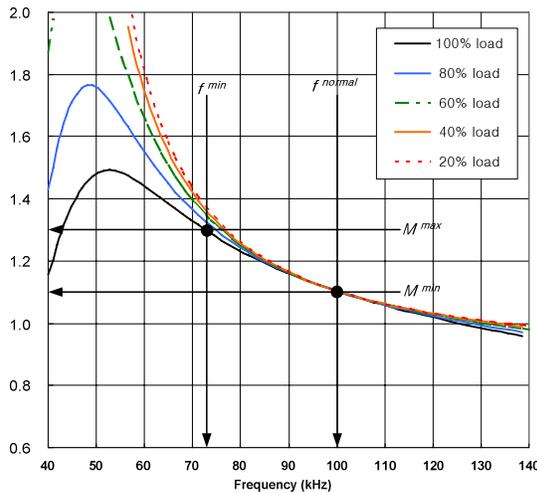
**Figure 23. Gain Curve of the Final Resonant Network Design****[STEP-8] Select the Resonant Capacitor**
