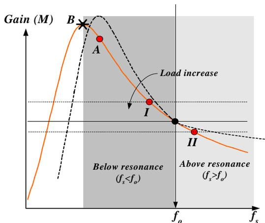
Figure 10. Operation Modes According to the Operation Frequency
